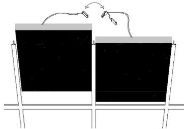
Connect a Jumper Jack to the first panel and connect it to the next panel. Up to twelve twilight Panels can be connected together in any configuration. If your installation requires more than twelve twilight Panels, then add an additional Driver and Leader Cable. **Note:** Do not exceed the capacity of the switched circuit.
