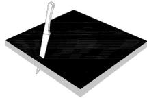
If necessary, cut border with knife. Make sure to cut the Drop In Panel from the face side along the marked lines. Make sure to make your cuts straight up and down and not at an angle.
