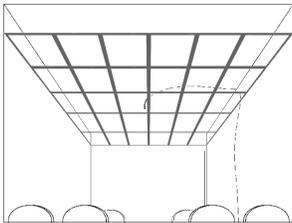
Based on site conditions and project design, generally you will have two options for power. The first and recommended way is using a Remote Driver and pre-installing an Twilight Leader Cable, or pre-wire an 18 AWG wire. Second is to plug the Driver into a switched outlet located above the ceiling. ***As always, check and observe local building codes.***
