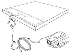
Connect the first panel to the Leader Cable. Inspect the front of the panel to see that the stars are illuminated.
