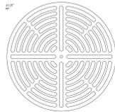
This template is a universal marking guide and cut-out stencil used for marking the center of a down-light, vent, speaker, or any hole that needs to be marked and cut in an Twilight Panel.
