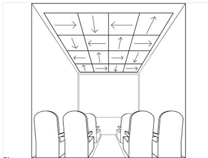
Each panel is marked with an arrow on the back. This arrow indicates the panels orientation. Every panel gets rotated one quarter turn in order to provide a more random starry night experience.
